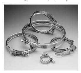
V-Band Couplings eliminate the need for cumbersome bolted flange designs and costly welded flange designs. Because V-Band Couplings can be easily assembled and disassembled, they are often used on equipment that requires frequent service or maintenance. Typical V-Band applications include pumps, engines, exhaust systems, filters, and food and chemical processing equipment.
